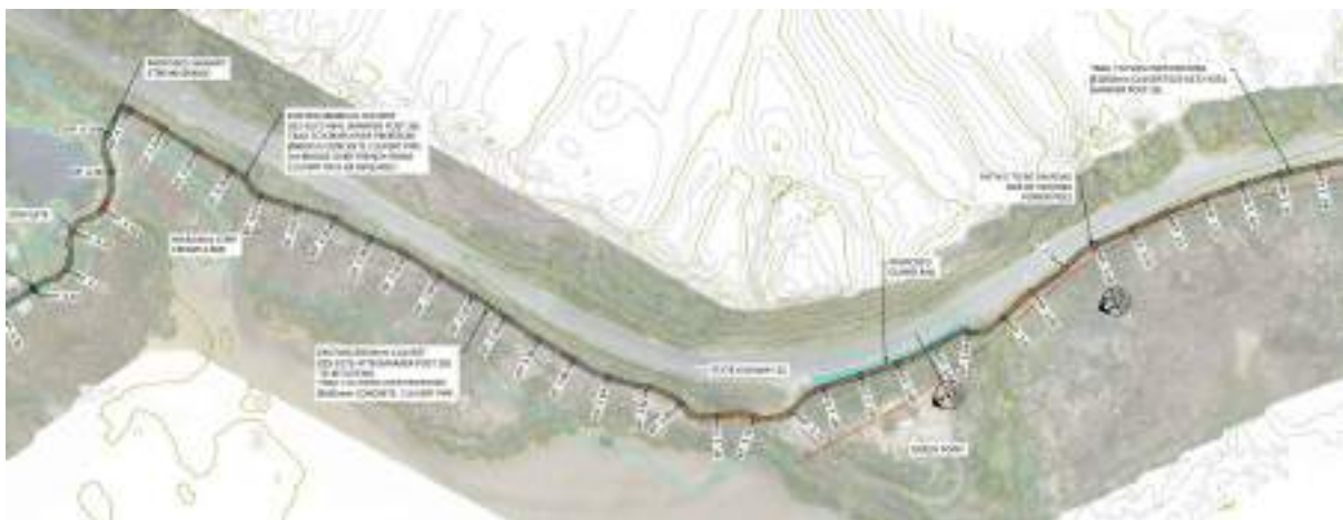
Figure 12: Trail set out from KP: 3.44 to KP: 4.22. Guardrail shown as pale blue between KP 3.64 and KP 3.72.
